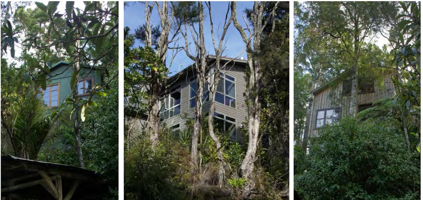
Darker building colours with a low reflectivity rating ensure that buildings blend with the bush setting and do not stand out, making them 'visually recessive'.
