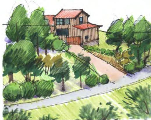
✗ Driveway runs straight up the contour necessitating earthworks.
