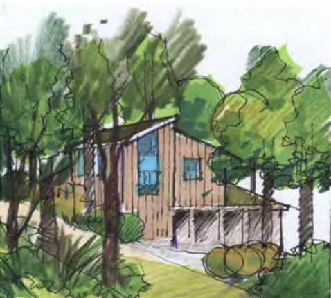
✓ Articulation of elevation and varied roof profile reduces building scale.
