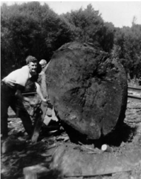
Figure 11. Shifting kauri log with timber jack, 1935
