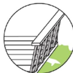
Timber handrail for safety from falling as required by the New Zealand Building Code
