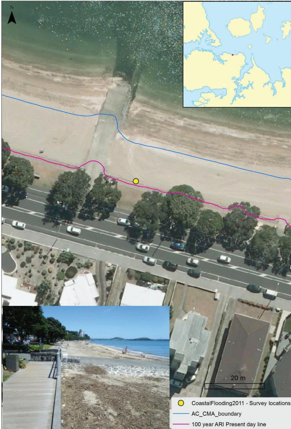
**Figure 8-9: Verification of present-day 0.01 AEP (100-year ARI) storm-tide line against surveyed location of maximum flood incursion during 23 Jan 2011 storm-tide, at Kohimarama.**
