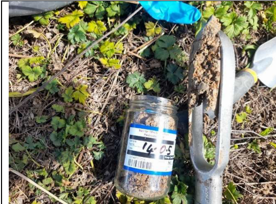
Image 7: Silty clay collected at test location 14 at 0.5 m depth.
