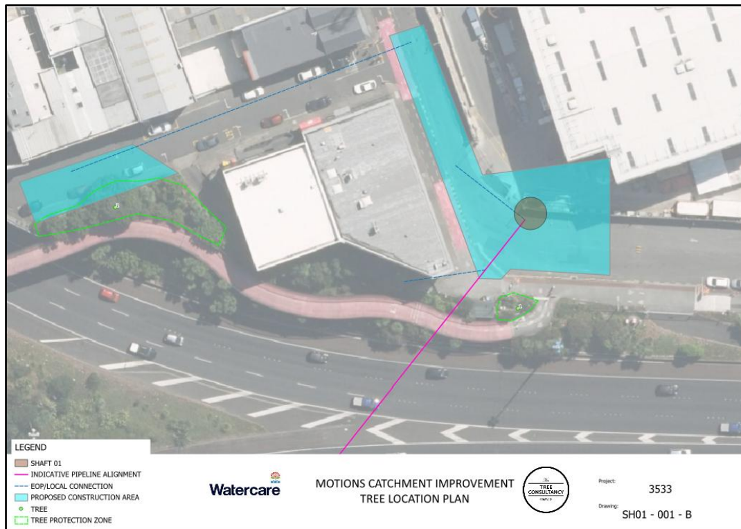
Figure 2: The proposed location for Shaft 1.
