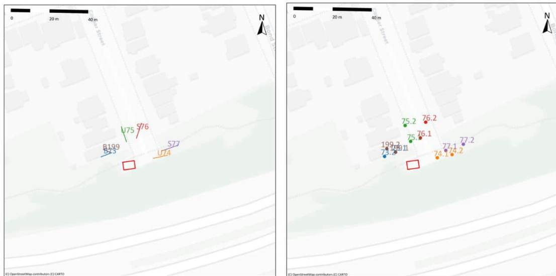
Appendix Figure G45: Location of the proposed excavation, and point pairs used to calculate settlement and differential settlement.
