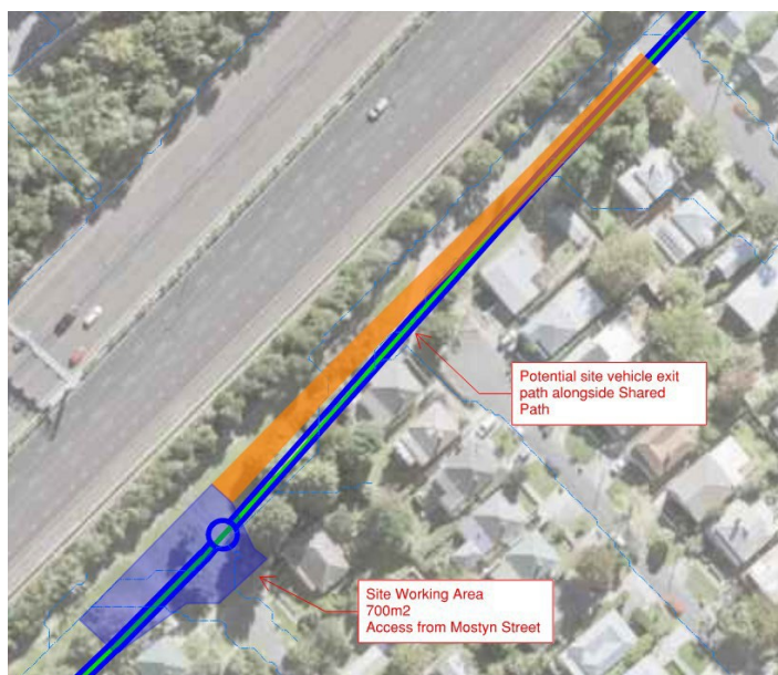
Figure 5 Working Area for SH03.
