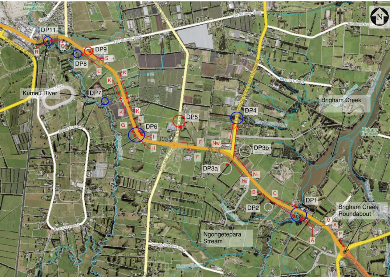
Figure 5: Location of proposed and decommissioned discharge points
