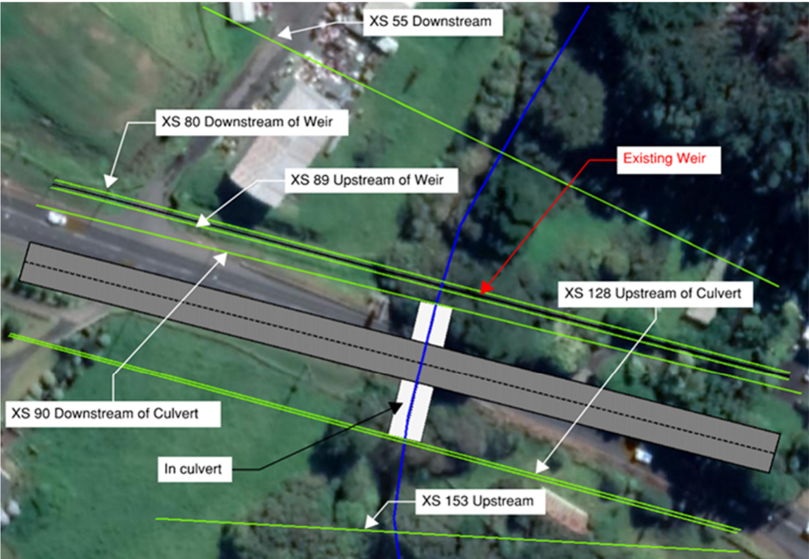
Figure 9: Image showing set out of HEC-RAS model and locations of the cross sections reported.
