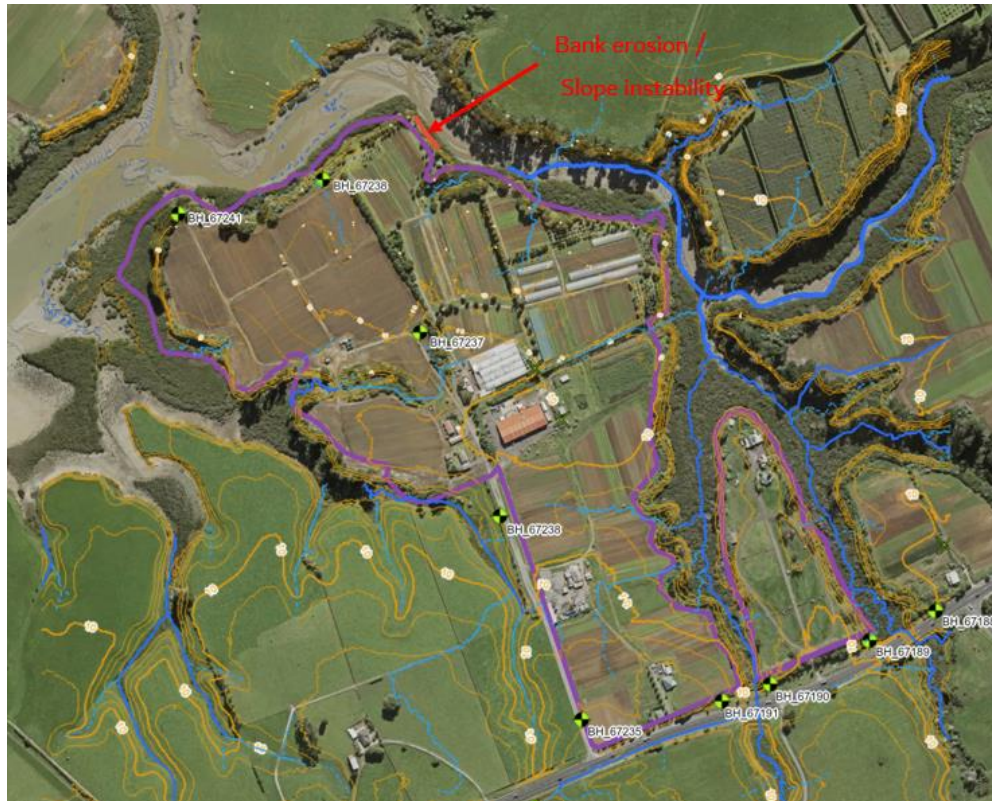
Figure 3: Location of bank erosion section
