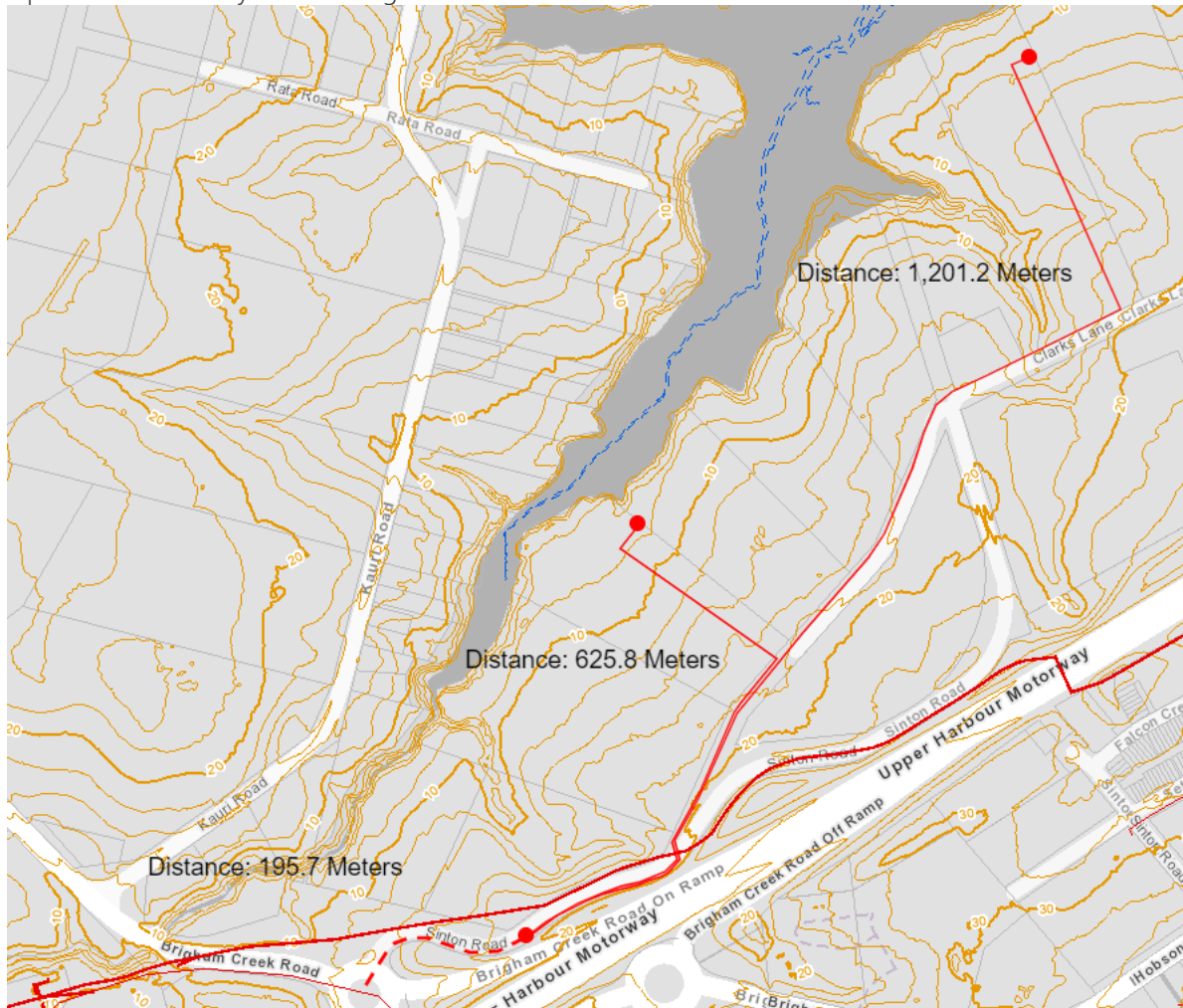
Figure 9: Option 3 – Connection to Brigham Creek WWPS.
